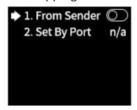
In the submenu, press the knob/OK to set the sender as the connection source. Then select **Set By Port** to enter the submenu, in which you can choose the Ethernet port that needs setting mapping, and set the offset values of X and Y, and the width, height, row number, column number and link type of the corresponding cabinets. Finally select **Save** to save the mapping.
