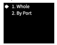
Output shift contains two selections: Whole and By Port. On the submenu of Whole, you can rotate the knob to set the row starting point (X) and the column starting point (Y) of the whole image and then save the setting; on the submenu of By Port, you can respectively set the row starting point (X) and the column starting point (Y) of the image of the 20 Ethernet ports, and then save the setting.
