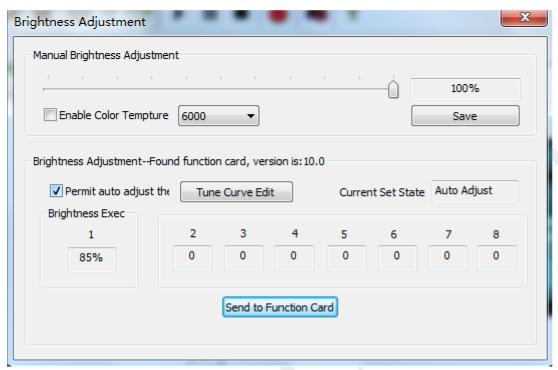
After select [Permit auto adjust], and send to function card, the function card will adjust the brightness of LED screen throw the data got from brightness sensor. The number in [Brightness Executed] is the current brightness level of Led screen.
