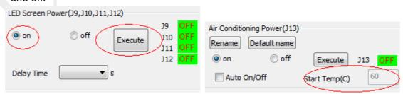
J9~J12 are controlled at the same time, J13 and J14 should be controlled throw temperature.
