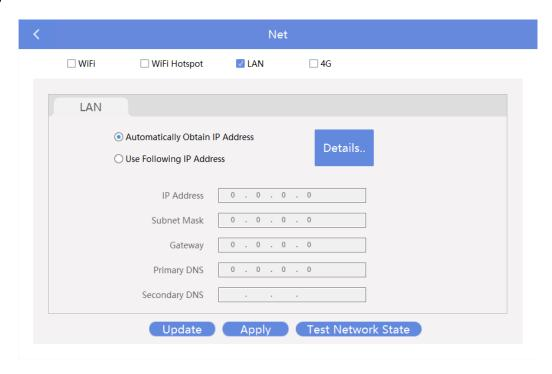
Take LAN as an example, the player will automatically obtain the IP address after connecting to the Ethernet cable.
