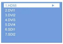
Enter the cropping interface of "HDMI", "DVI1/2/3/4", or "SDI1/2", then press the knob/OK to turn the crop on or off. If it has been enabled, set X, Y, width and height of the input signal with the knob, then save the data.
