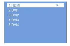
Enter the EDID setting interface of "HDMI" or "DVI1/2/3/4" (take "HDMI" as an example). Rotate the knob to select conventional resolution; or set width, height and frame rate by knob in the "Custom" option.
