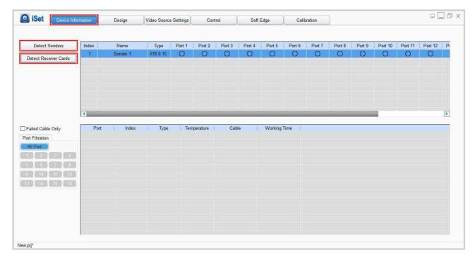
2. Click [Detect Receiver Cards], the port, index, type, cable status and other information of receiver cards will be showed in the display area. Please check corresponding cable if the numbers of receiver card are inconsistent with actual status.
