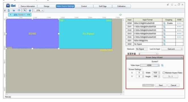
Similarly, select the input signal source of screen 2 in [Video Input], then scale and crop the screen 2, then click [Finish] to complete the screen setup.
