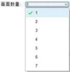
Take 2 (number of layers) as the example, select [Number of Layer] for 2, and the screen setup wizard will pop up. Select the input signal source of screen 1 in [Video Input], scale the screen 1 in [Screen Settings], click "\sum\_" to crop the screen 1, then click [Next] after completing.
