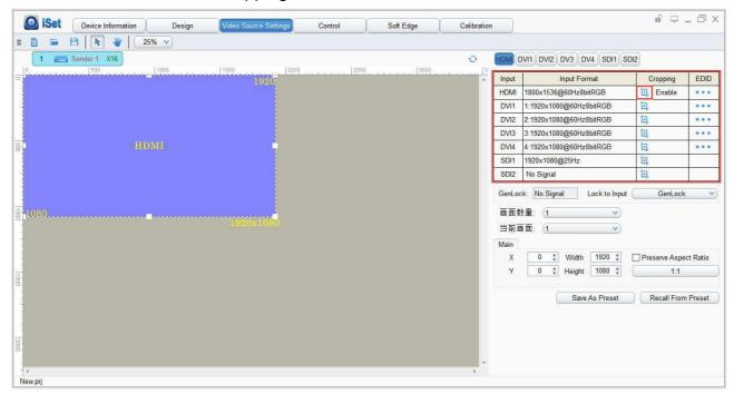
In the cropping interface, check out [Crop], set the row starting point (X), column starting point (Y), width (W) and height (H) in [Cropping Information], then the cropping will be completed.
