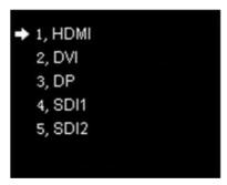
Enter the cropping interface of "HDMI" or "DVI" or "DP" or "SDI1" or "SDI2", press the knob/OK to turn on/off crop. If it has been enabled, set x, y, width and height of input signal by knob then save the data.
