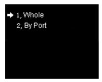
Output shift includes two ways: "Whole" and "By Port". In the setting interface of "Whole", you can rotate the knob to set x and y of the whole image and save it; in the setting interface of "By Port", you can set x and y of the image of each net port respectively, then save it.
