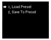
In the submenu, 16 preset parameters can be saved, and every preset parameter includes all parameter information of source setup (signal source, PIP, scaling, cropping, picture adjustment), users can also directly load the saved preset parameter to display the image according to needs, and don't need to set up all parameters again.
