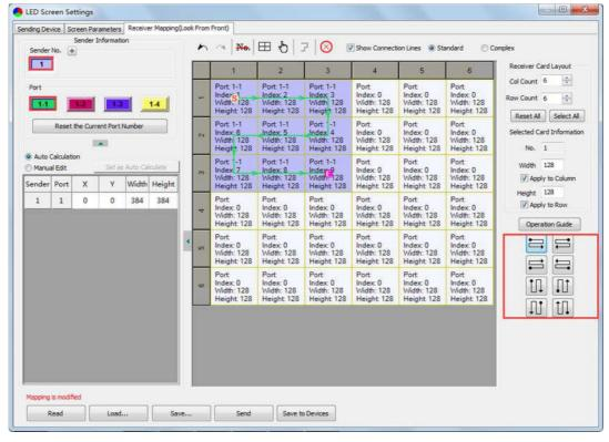
**Note:** As the cabinets have multiple and different specification (that is the inconsistent capacity of the receiving card), you can select the different one to adjust separately after completing setting.
