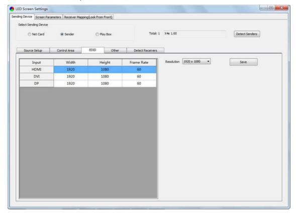
Click the dropdown button to display the resolution list to select the mainstream resolution, and you can also customize the sender resolution, by setting the width/height and frame rate.
