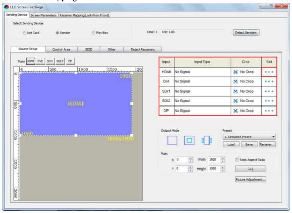
In the cropping interface, check **[Crop]**, and set X, Y, width and height in **[Cropping Settings]**, then the cropping setting is auto saved.
